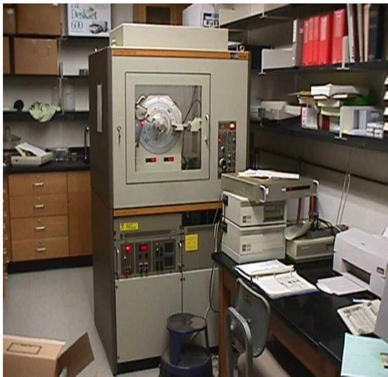
Siemens D-500 X-Ray Diffraction System
